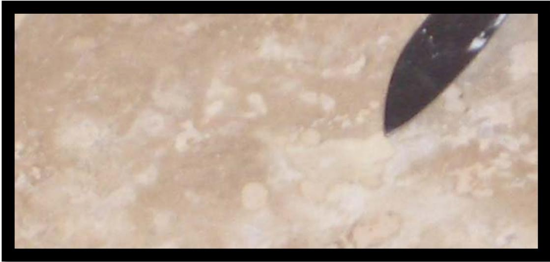
**Tip:** If the void is large, sometimes the amount of water held in the void is not sufficient to moisten the grout. When this occurs simply dip the tip of your finger into tap water. The surface tension of water will cause a half-drop to be attached to your fingertip. Carefully place this small amount of water onto the center of the grout until moist. Too much water and you will need to start over. Coaching is available from your account representative or call Durango Stone™ at 602-438-1001.
