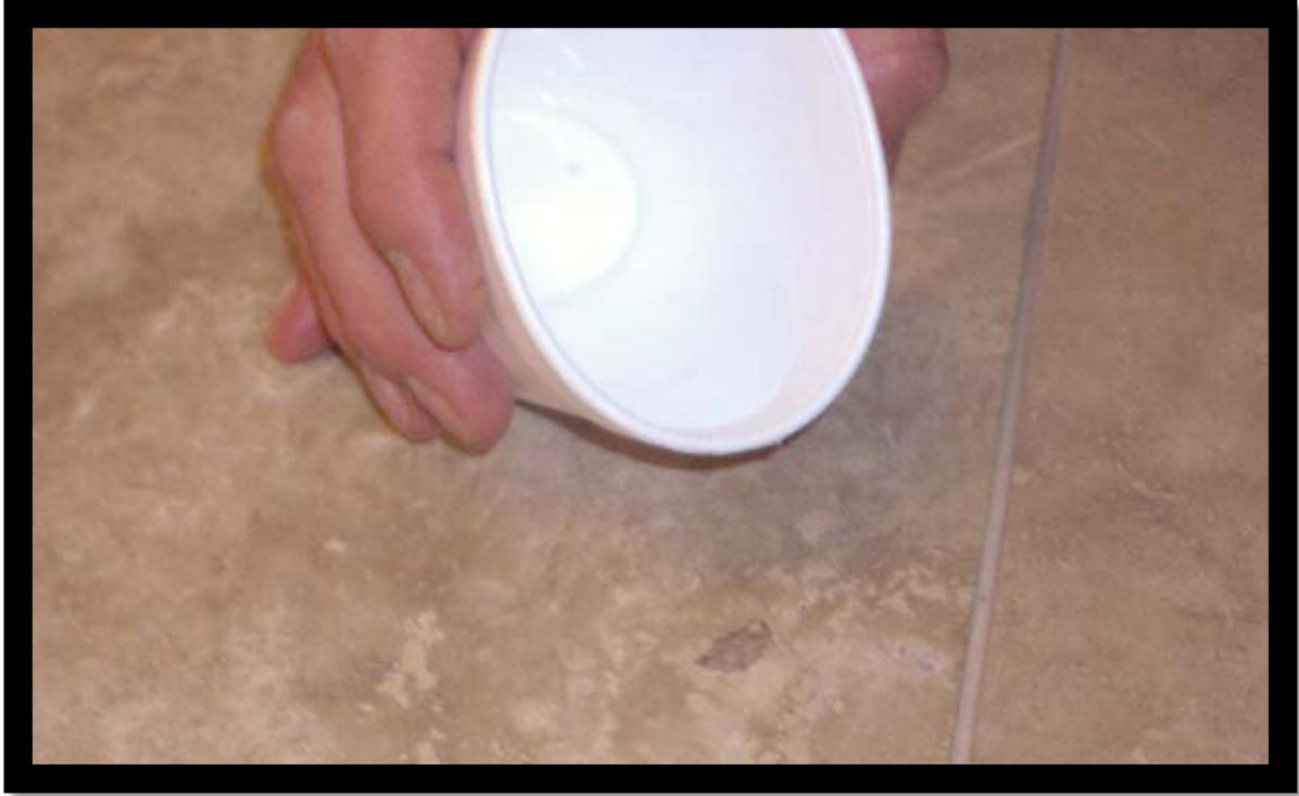
**Step 3:** Fill hole with tap water. Pour enough water into the hole until water will remain in the hole for a second or two.
